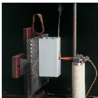
Apparatus for testing heat resistance (850° C) GWT.
