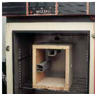
Cabin for age acceleration test.
