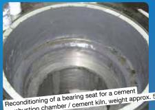
combustion chamber / cement kiln, weight approx. 500 t
