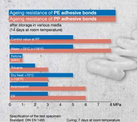
Adhesive surface: 12,5 mm x 25 mm Testing speed: 10 mm/min Adhesive thickness: 0,2 mm
