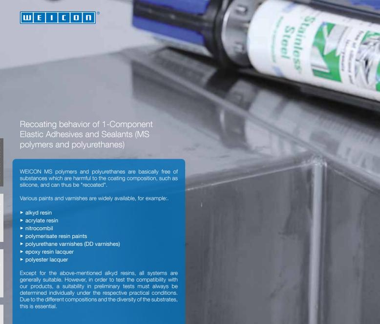
It also must be taken into account that not only the immediate first paint layer or lacquer layer, but also all possible intermediate lacquers or top lacquers, have an effect on the bonding and / or sealing.
