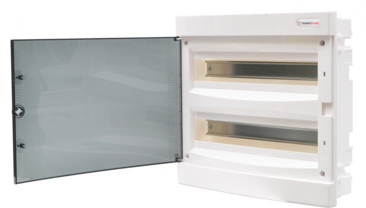
Enclosures Flush mounting - IP40 - 36 Modules (2x18) 392 x 357 x 106 mm
