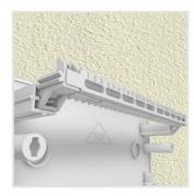
Isolated terminal inside the plastic box, which is made of self-extinguishing material with glow wire test up to 960 °C and thermostable up to 120 °C.
