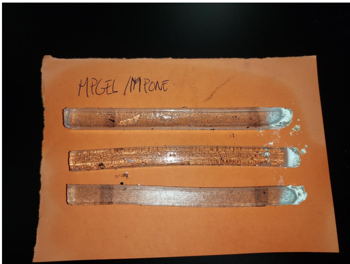
Appearance of the samples after the test as per EN 60695-11-10 Horizontal Flame Test
