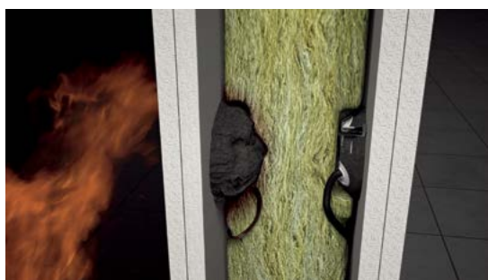
Demonstration of the behavior of a fire resistant instrument box.
